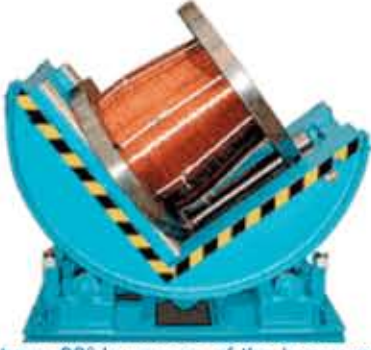
The reel turns 90° by means of the heavy mechanical tilting unit.
