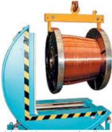
Placing the take-apart process reel on the reel tilter with a jib crane and the exact adjusted lifting device
