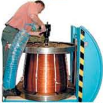
Bolts are removed using air wrench
